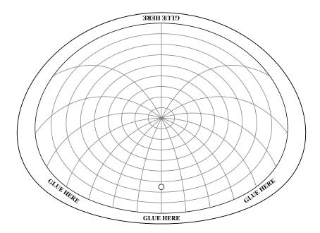
This grid of lines can optionally be printed onto transparent plastic and glued into the cut out window in the planisphere's body to show the altitudes of objects in the sky, and their directions.
