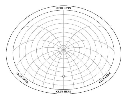
This grid of lines can optionally be printed onto transparent plastic and glued into the cut out window in the planisphere's body to show the altitudes of objects in the sky, and their directions.
