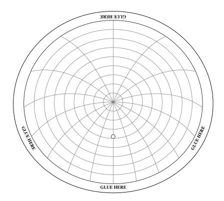
This grid of lines can optionally be printed onto transparent plastic and glued into the cut out window in the planisphere's body to show the altitudes of objects in the sky, and their directions.
